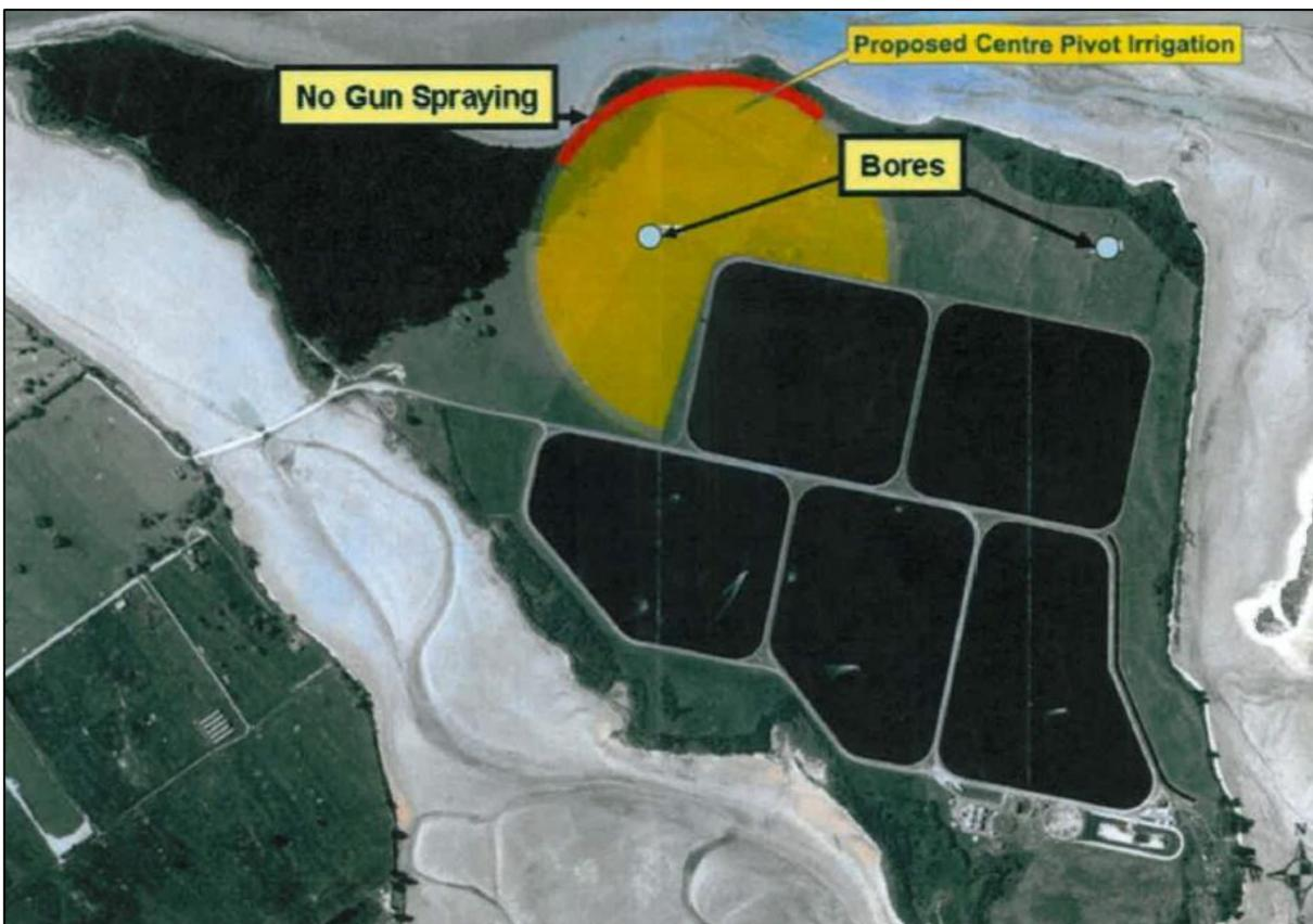
**Figure 2.** Location of Wastewater Irrigation Area (shown in Yellow) and Monitoring Bores.
