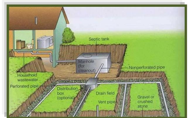
Cutaway section of a generic wastewater system
